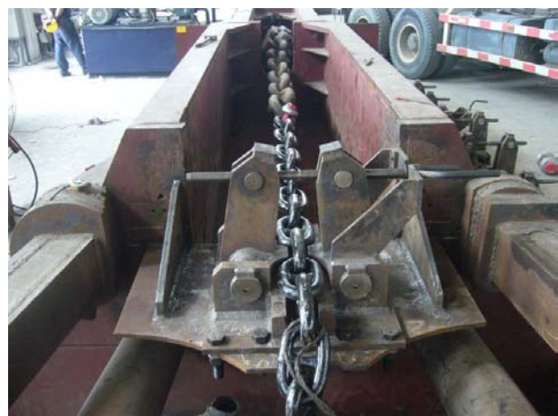
Pull Load Test
